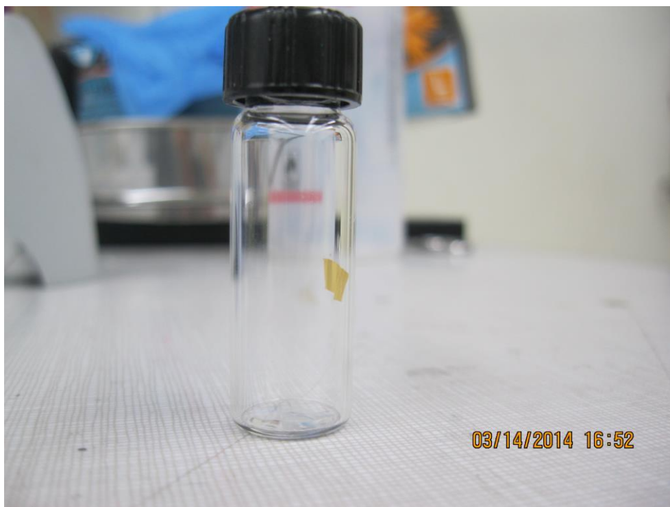
Figure 6-3 Au nanohole membrane attached on the inner wall of a glass bottle.
